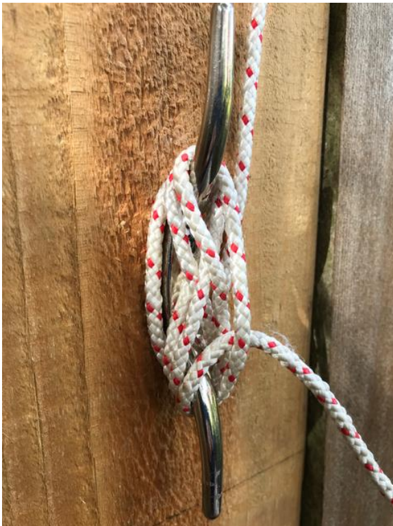
A cleat is a convenient way to anchor a rope under tension.
