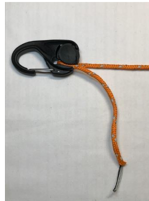
The Cam-Jam has a ratchet cam to hold the rope. The end of the rope is passed through the hole, then pulled into the cam. Pulling the rope back toward the antenna tightens the rope. Pulling it toward the camera releases it.
