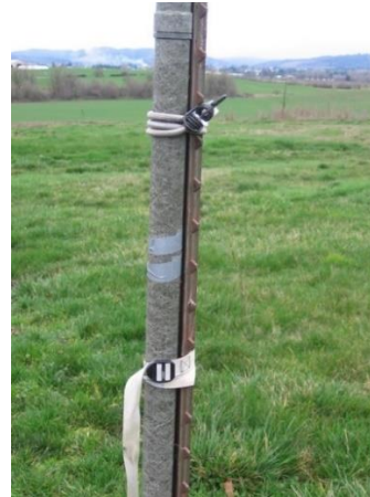
A bungee cord (top) and nylon strap (bottom) are used to secure the base of a mast to a fence post.
