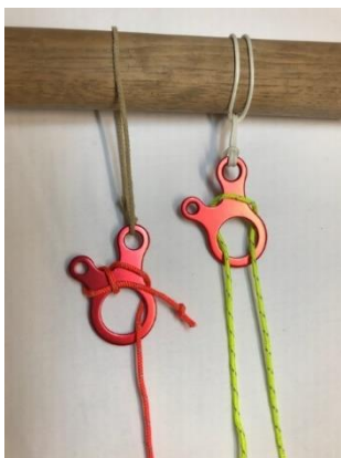
Red aluminum "snail" tensioners can be used several different ways. Note the pre-tied loops used to attach them to the anchor.
